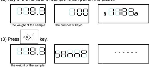
(4) When the scale is stable, it is finished for sampling and enters in the counting mode.
